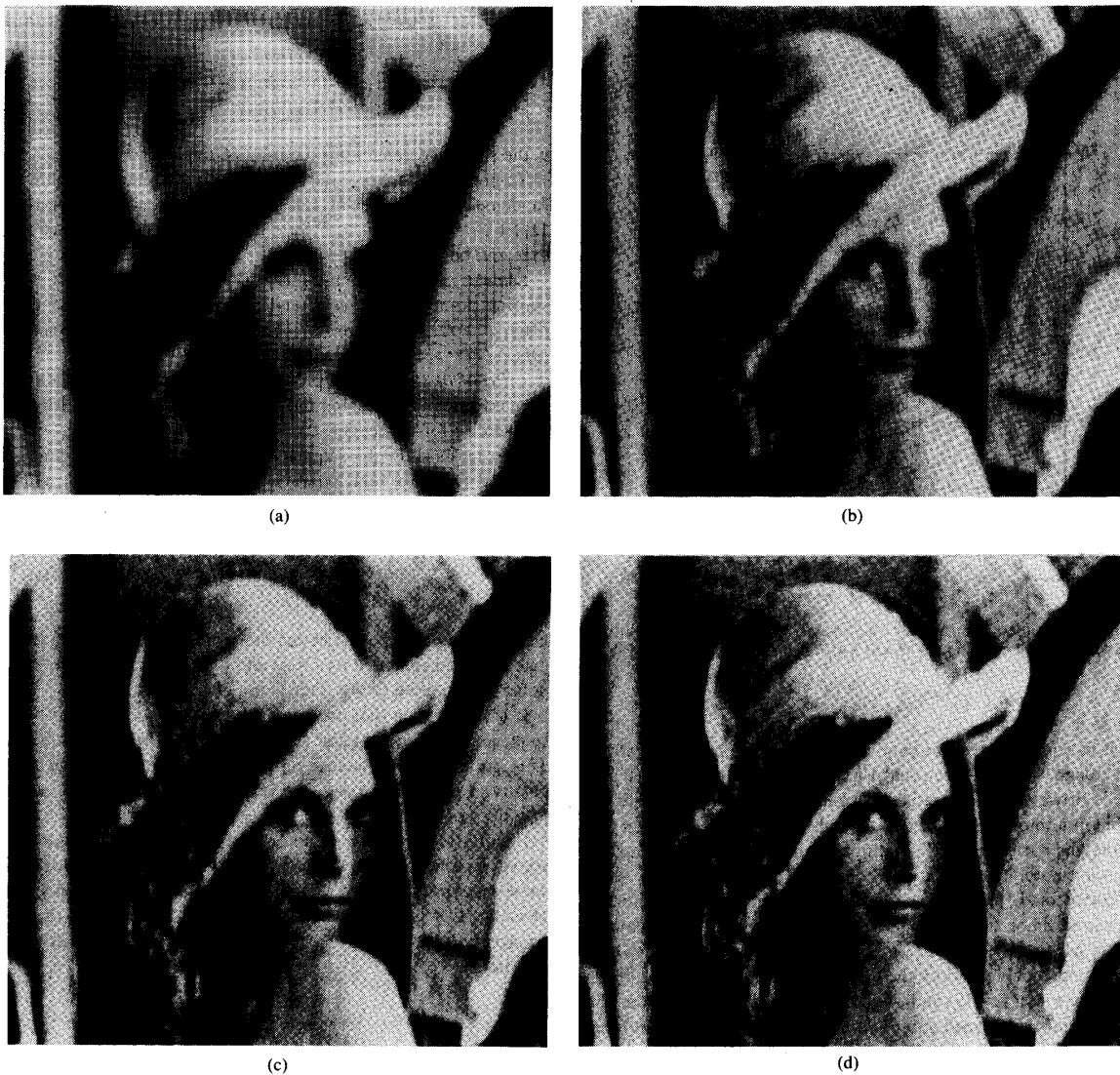
Fig. 6. (a) Image degraded by an 11 \times 11 ill-conditioned low-pass filter and a 40-dB SNR; MSE = 674. (b) Image restored by the one-step Wiener filter, MSE = 328. (c) Image restored by 25 iterations of the iterative Wiener filter; MSE = 277. (d) Image restored by 25 iterations of the additive correction method; MSE = 236.
